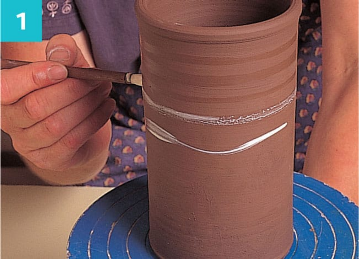
1 Stripes of wax are banded onto a leather-hard cylinder as a resist, using a proprietary brush wax, which washes off brushes and is easier to manage than hot wax.
