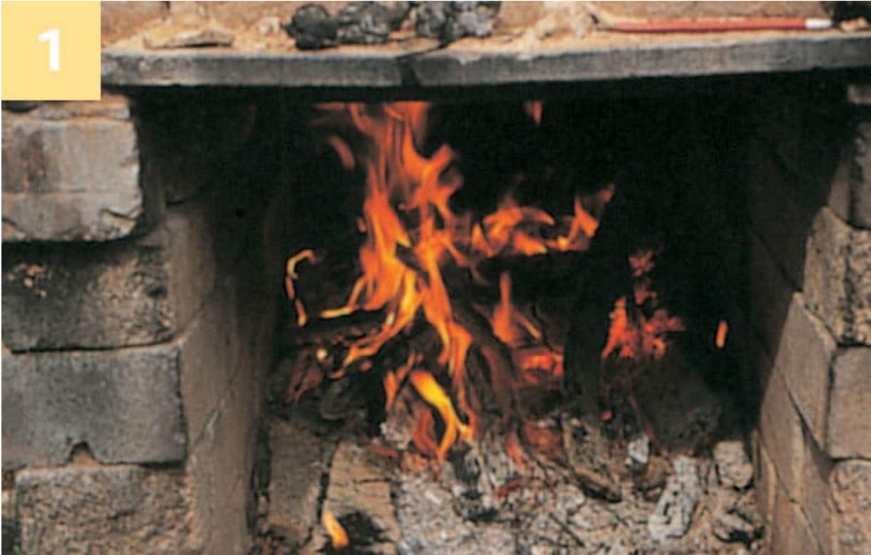
1 Flames are drawn from the firebox underneath the chamber and back through the pots, exhausting through the chimney.
