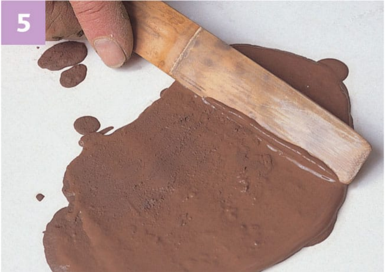
5 Pour the sieved slip onto a plaster bat and smooth it out. The slip will stiffen fairly quickly and will need frequent turning on the bat to stop it from hardening too much.
