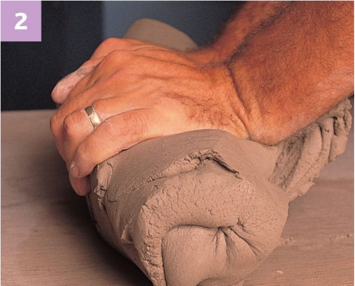
2 The kneading process should be carried out several times to ensure that the whole clay mass is thoroughly mixed.
