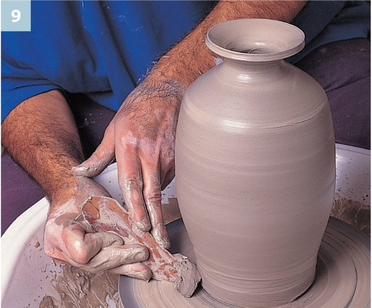
9 With the sharp point of the rib, trim off the excess clay at the base, until it is the approximate final shape. Cut the bottle from the wheel-head with a wire, and leave to set up on a wooden board before trimming the foot ring (see page 60 ).
