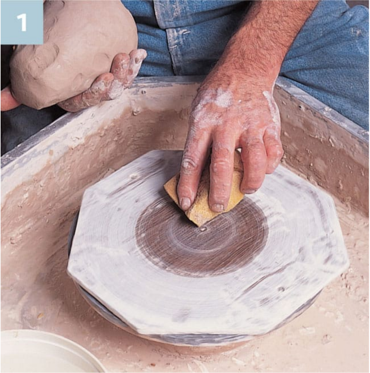
1 The wheel-head needs to be damp to help the clay adhere, so wipe it with a damp sponge if it is dry. Take care not to wet it too much, however, or the clay will slide off as the wheel gathers speed.
