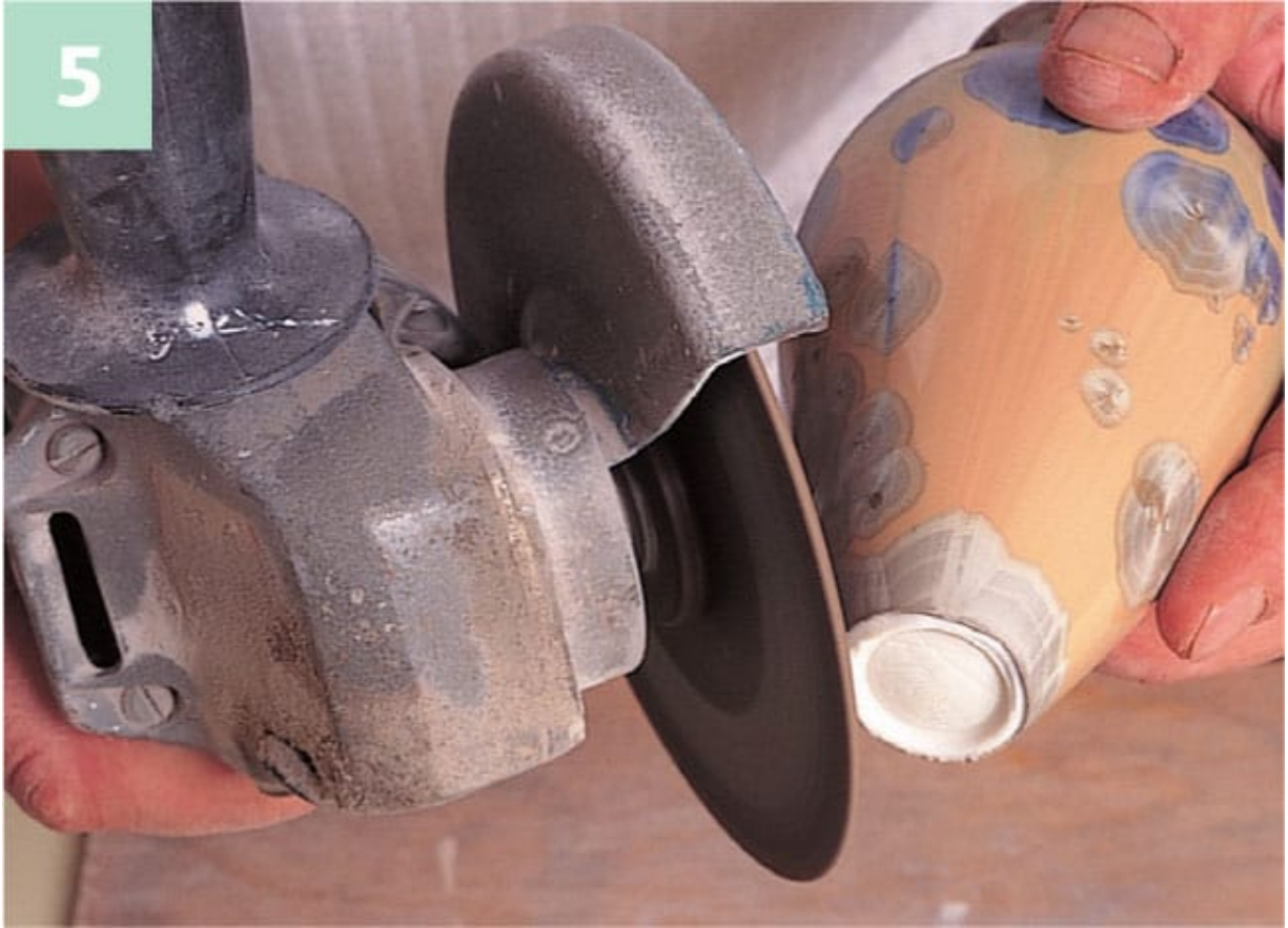
5 The sharp edges are ground off with an angle grinder.
