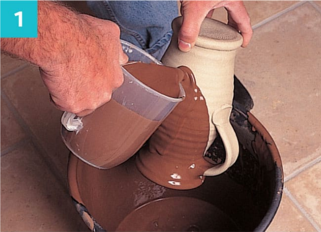
1 Slip is poured down one side, then allowed a few moments to drain.
