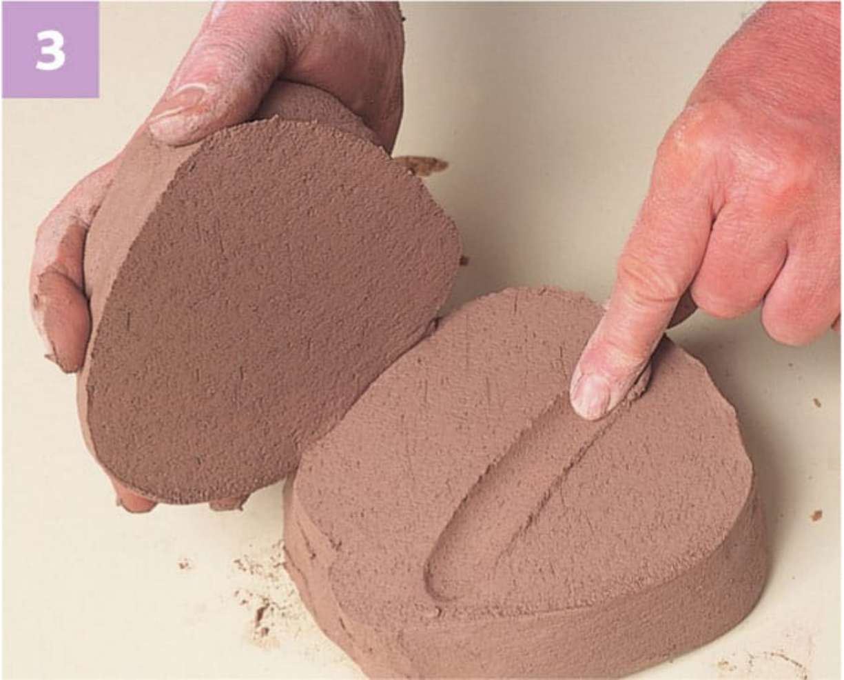
3 Use a wire to cut the lump in half and run your finger across the cut surface to check that the grog is evenly dispersed throughout the body.
