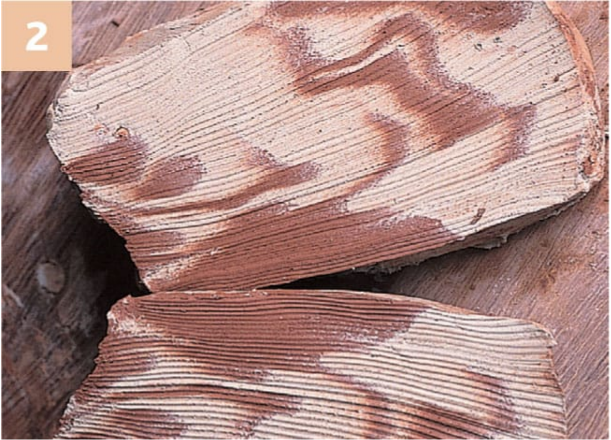
2 Slicing through the block of clays will reveal the extent to which they have blended together. Strong agate patterning is usually the result of a smaller ratio of the stronger color.
