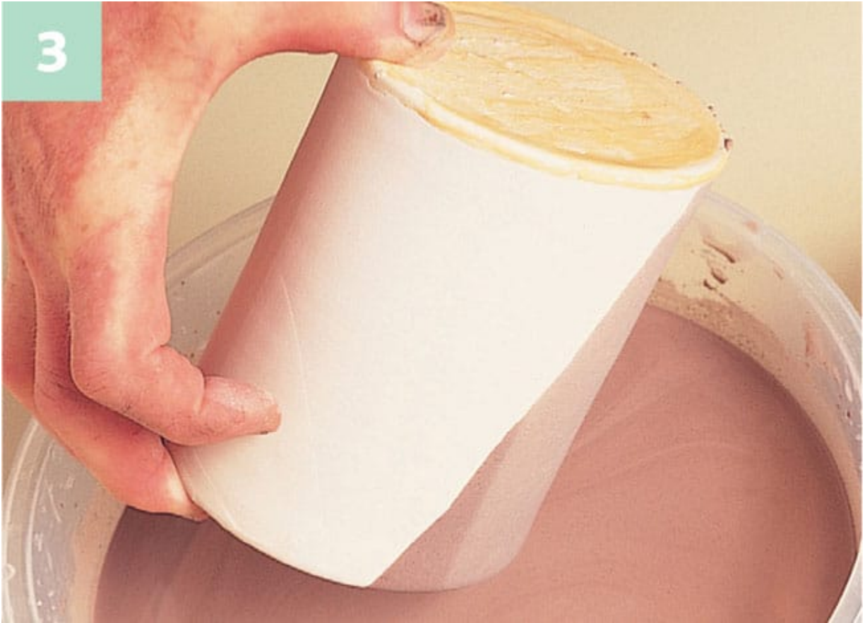
3 When the glaze is dry enough to touch, the pot is held and dipped the other way, overlapping the first glaze in the middle.
