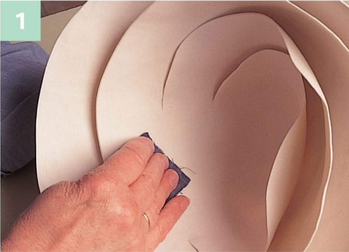
1 The bowl is fired to 2246°F (1230°C) without glaze and rubbed down with fine-grade wet-and-dry carborundum paper.
