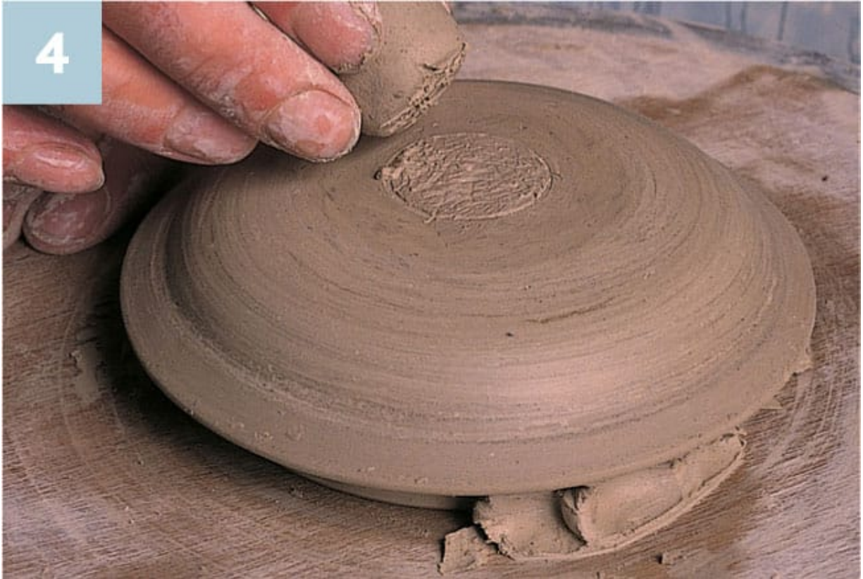
4 Lids thrown in an inverted position will normally require some form of knob or handle. This can be a section of pulled or extruded handle, but an alternative is to throw a small knob directly onto the lid.
