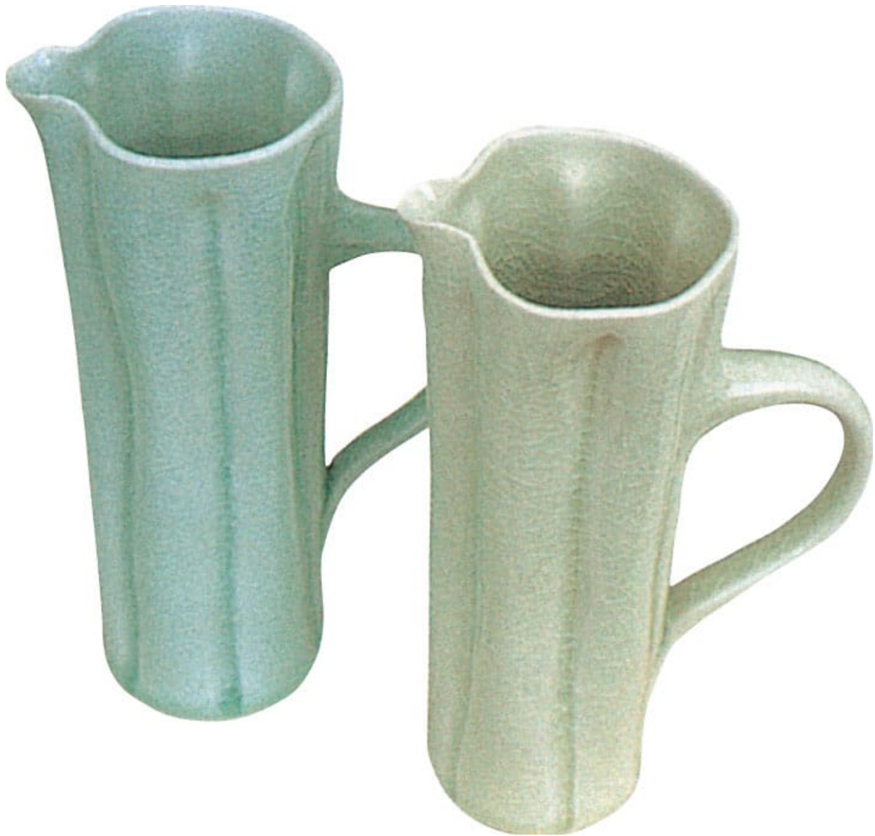
Two Tenmoku-glazed mugs showing a difference in color from firing: oxidized (left), and reduced (right).
