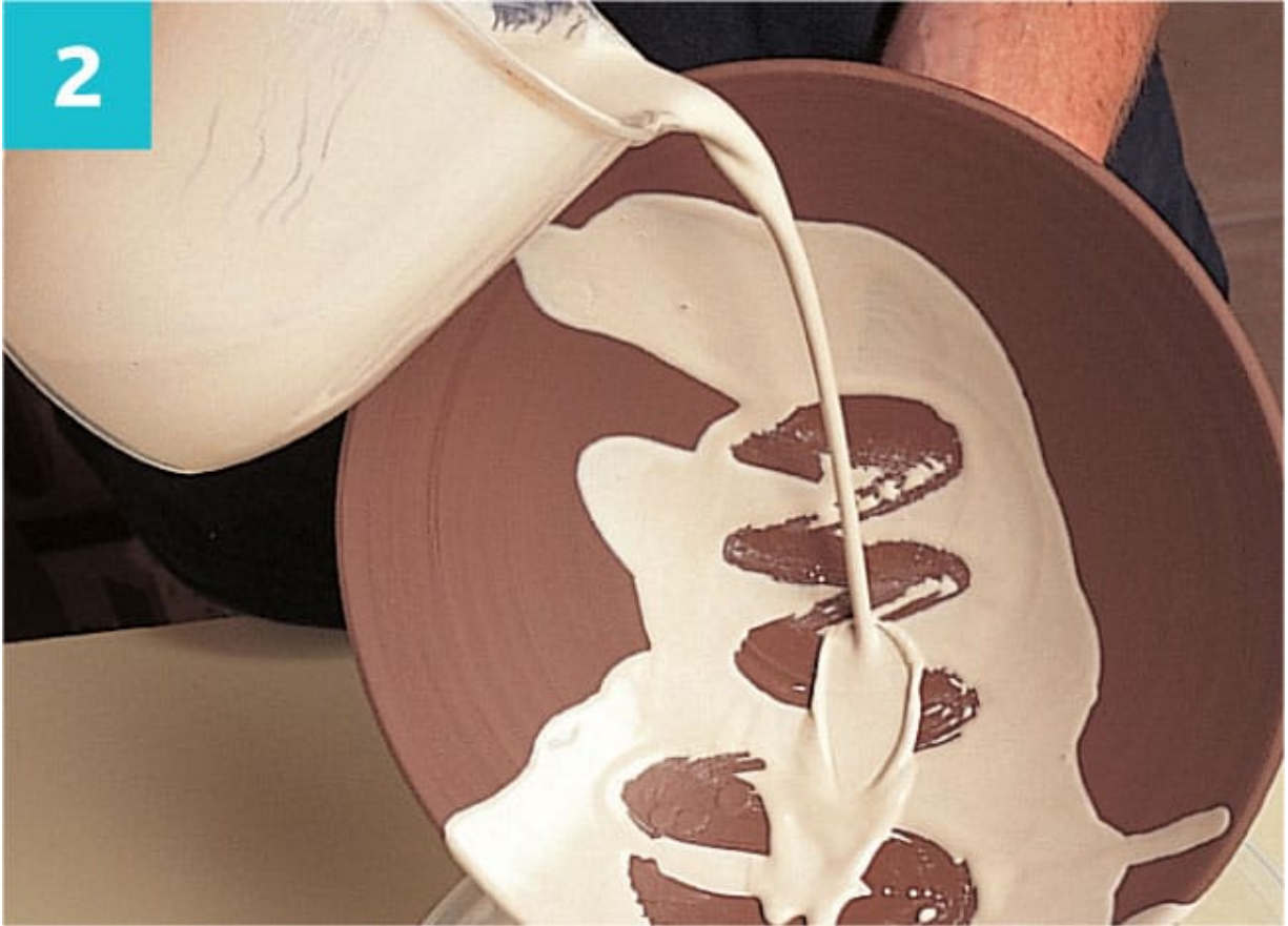
2 White slip is gently poured over the bowl, which is held at an angle to prevent the slip pooling in the center.
