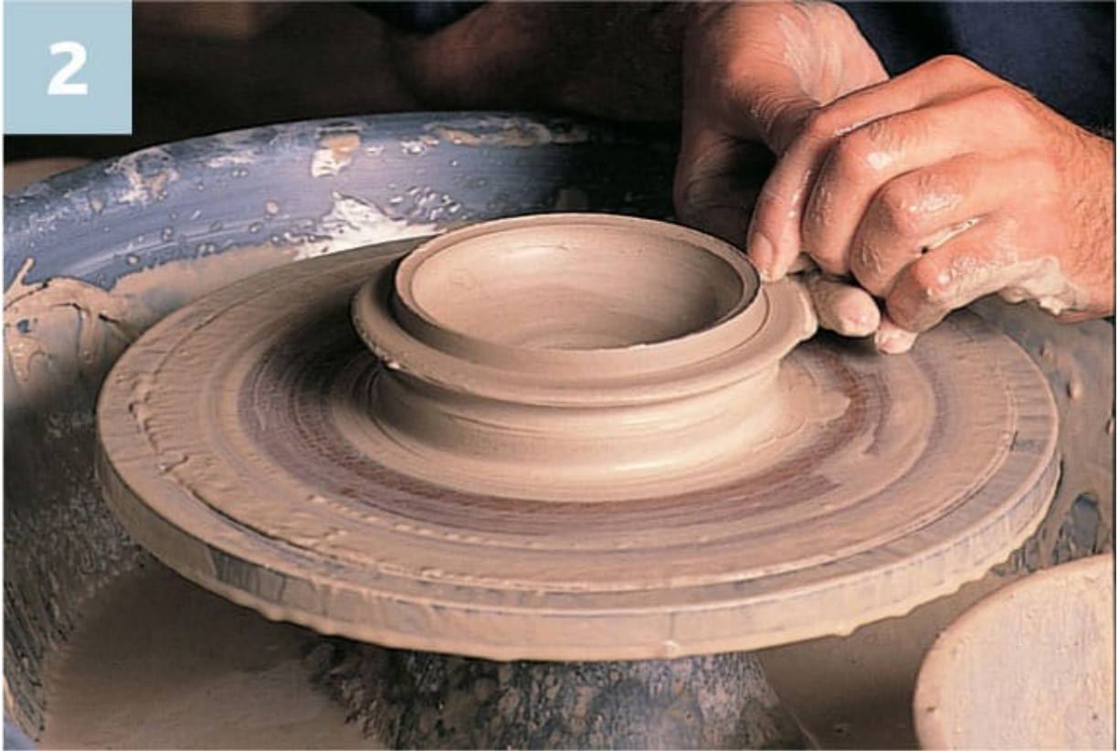
2 To make a flange lid, begin by compressing the rim to thicken it. Determine where the flange will form and split the resulting thickened rim with your fingernail. Press down steadily on the split section.
