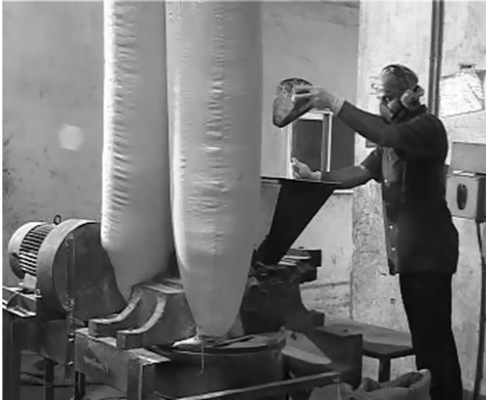
FIGURE 3.7 Pulverizer for size reduction of herbs. Photo courtesy: Nagarjuna Herbal Concentrates Ltd, Kerala ( www.nagarjunaayurveda.com ).
