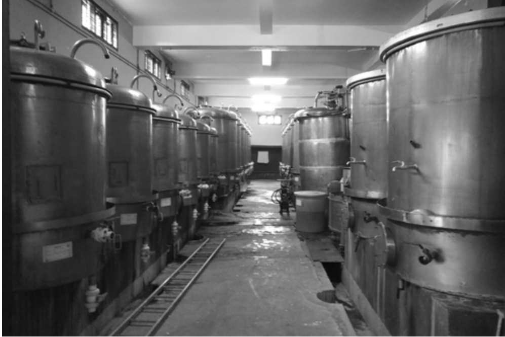
FIGURE 3.14 Modern brewing tanks in fermentation room. Photo courtesy: Nagarjuna Herbal Concentrates Ltd, Kerala ( www.nagarjunaayurveda.com ).
