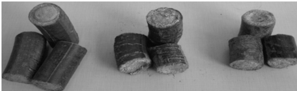
FIGURE 3.22 Briquettes made from feedstocks such as corn stover, switchgrass and prairie cord grass. Reproduced with permission from Karunanithy et al. (2012).
