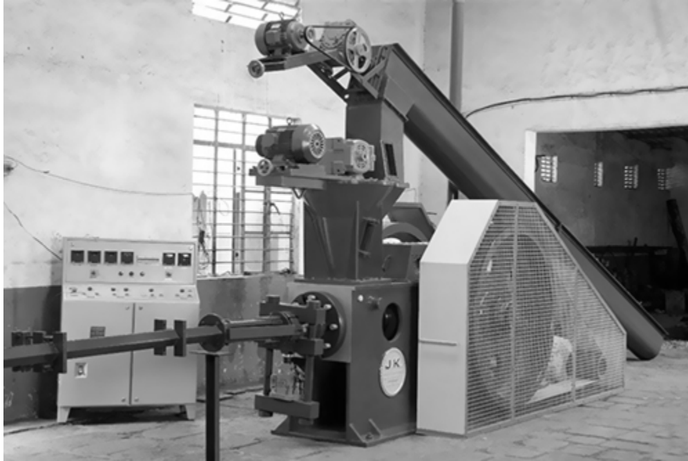
FIGURE 3.21 Briquette press used in compaction of powdered raw material. Figure of Jumbo Brq 9075 briquette press. Reproduced with kind permission of Jay Khodiyar Machine Tools, Rajkot, India ( www.jaykhodiyar.com ).
