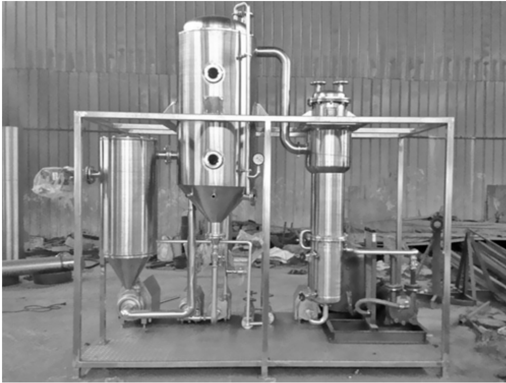
FIGURE 3.10 Forced circulator evaporator for concentrating kvātha . Photo courtesy: Nagarjuna Herbal Concentrates Ltd, Kerala ( www.nagarjunaayurveda.com ).
