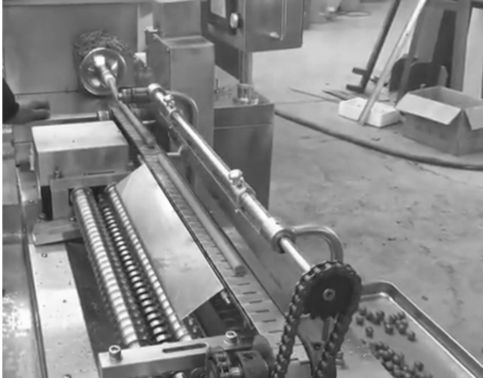
FIGURE 3.19 Pills rolling machine. Photo courtesy: Nagarjuna Herbal Concentrates Ltd, Kerala ( www.nagarjunaayurveda.com ).
