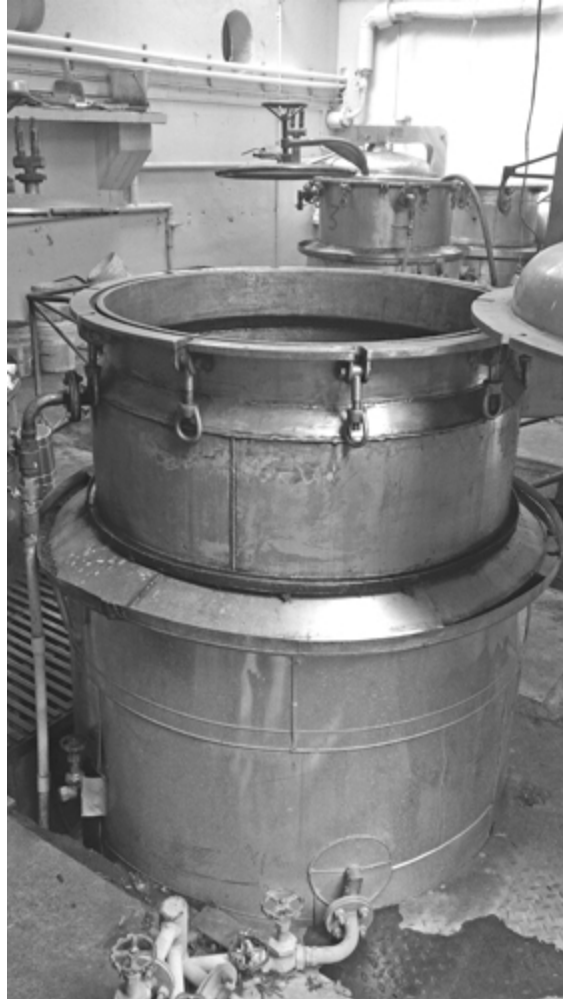
FIGURE 3.8 A drug boiler used in the manufacture of kvātha . Photo courtesy: Nagarjuna Herbal Concentrates Ltd, Kerala ( www.nagarjunaayurveda.com ).
