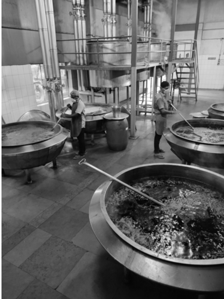
FIGURE 3.16 Avalēha being cooked in large steam-jacketed evaporators. Photo courtesy: Rajah Healthy Acres, Kerala ( www.ayurvedichospital.com ).
