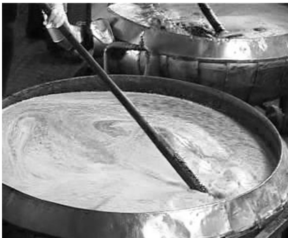
FIGURE 3.13 Steam-jacketed evaporators employed in production of medicinal lipids. Note froth on surface. Photo courtesy: Nagarjuna Herbal Concentrates Ltd, Kerala ( www.nagarjunaayurveda.com ).
