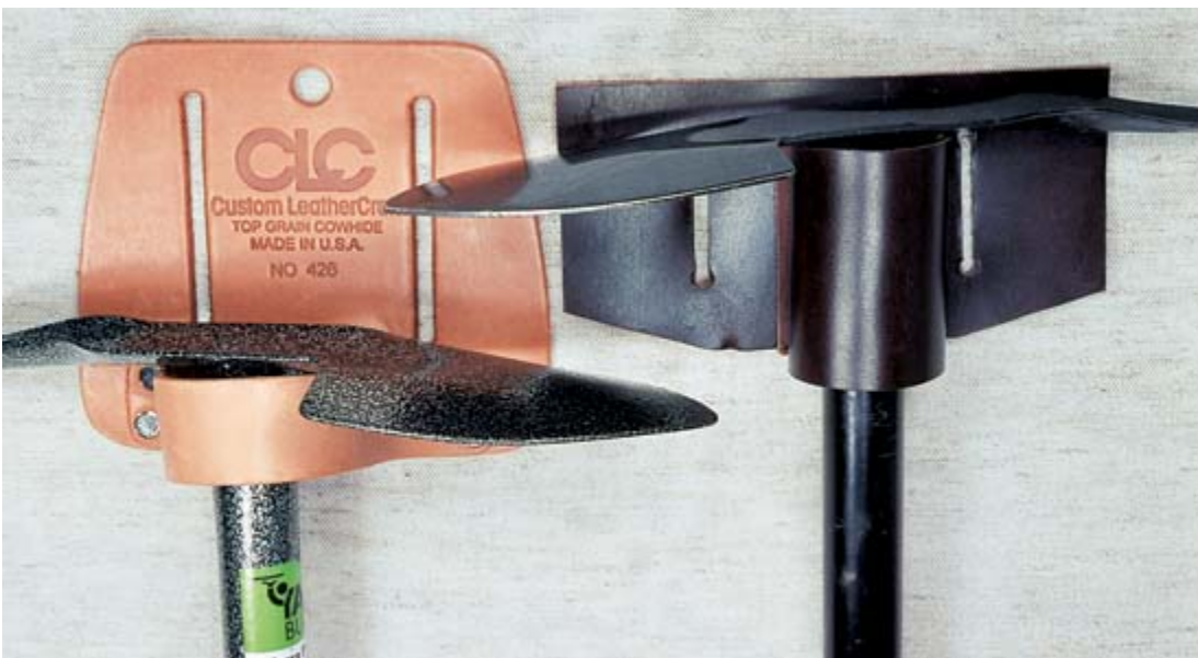
Spade-picks in sheaths. The one on the left is a standard sheath that is designed to hold a hammer (Custom LeatherCraft, Model #426). The spade-pick sheath on the right is one I built myself.
