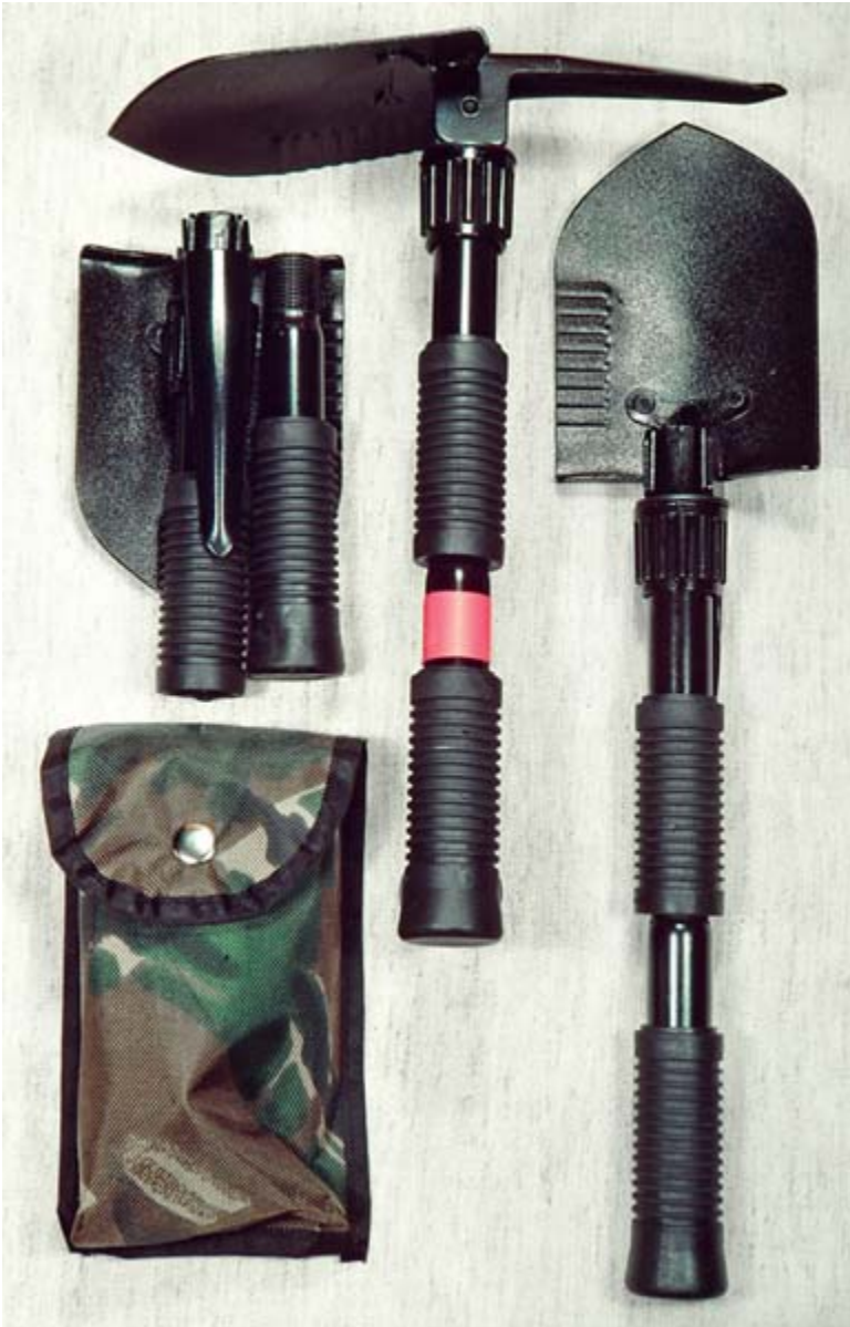
Folding shovel-picks: (left) folded shovel-pick and sheath; (center) assembled shovel-pick positioned for shoveling or picking; (right) assembled shovel-pick positioned for shoveling.
