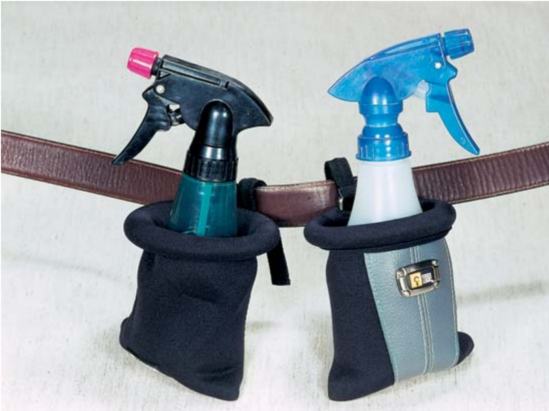
Spray misters in belted Catch-Alls. The Catch-All on the left comes with a hook-over-the-belt arrangement. I bent the hook on the Catch-All on the right to circle and fit more snugly on the belt. The shaped hook does not fall off the belt as you move around.
