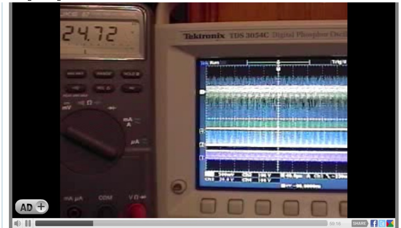
A now recorded 24 Volt battery bank voltage increase seen on the Fluke 87 from the starting voltage of 24.70 to 24.72 DC volts.
