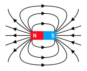
Both North (N) and South (S) poles are labeled on a magnet. The magnet force moves from the North poles to the South poles in a vacuum. A magnetic field around a magnet is formed .
