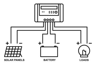
A power controller is known as a solar charge controller from the individual solar panels to batteries. For systems that use batteries, the device is essential. If it is overloaded, battery life can be reduced. For the same reason, too, the battery can be damaged. A solar load controller avoids such. The solar charge controller controls the battery voltage, and the circuits are opened so that charge can be stopped at a certain point when the voltage is present .
