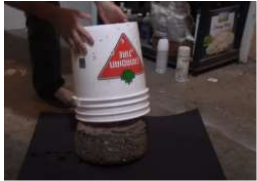
16. You can cut it now to your appropriate fire brick size to allow it dry quicker
