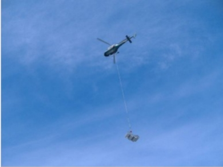
Slinging a load of diesel to the drill
