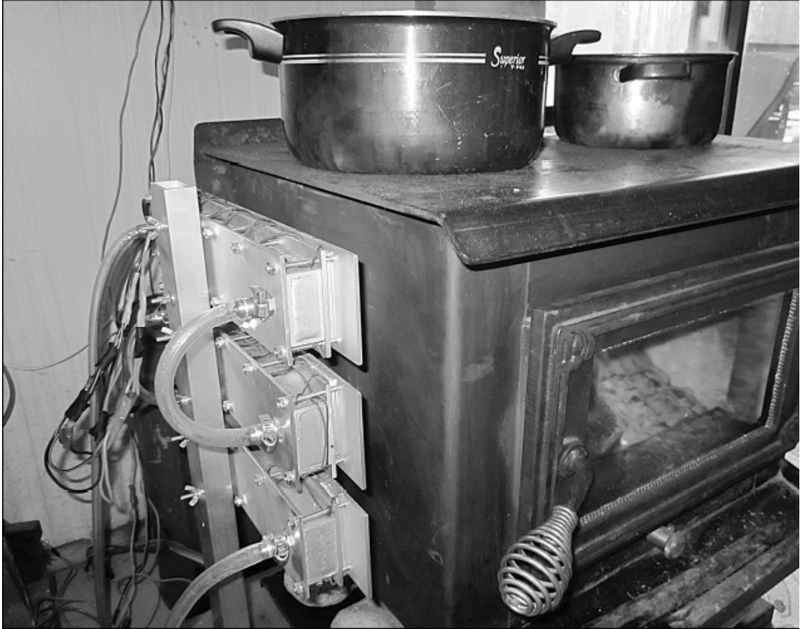
Thermoelectric modules on side of wood stove
