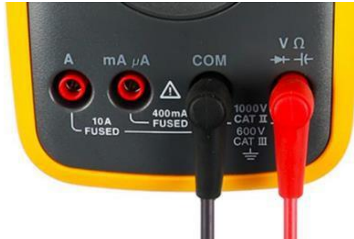
Input terminals of a multimeter (left: black, right: red)
