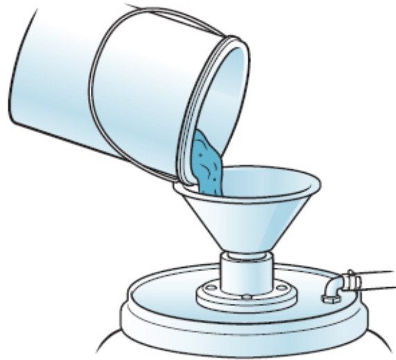
3. slurry poured into digester
