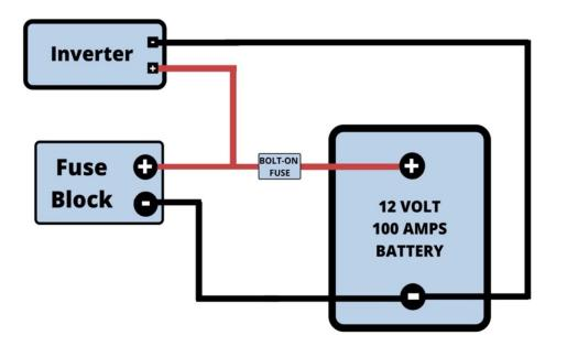
Connect the inverter to the battery bank directly using an inverter wiring kit (that might come with an inverter, or buy it separately), or choose the wire thickness the way I described above. Bolt positive cable to the bolt-on fuse, and after this connect the negative cable. Usually, the negative terminal (the wire that will be connected last) will spark when you connect the inverter, and it is normal. Now you can start the inverter and run the AC appliances by using the inverter.
