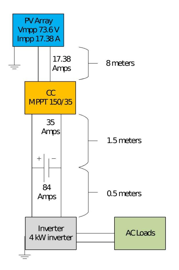
The formula used to determine the appropriate cable size is as shown below;
