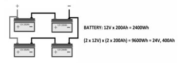
The day of autonomy refers to the amount of time (usually in days) that the solar power system can operate using battery power alone before you can use the generator. You can look at the amount of power you use daily or weekly to see how large the battery bank needs to last on days or weeks where there is no sunlight. Nevertheless, you need to remember that the more days you plan on using the battery alone, the larger and more expensive the battery bank will be. However, you do not want to
