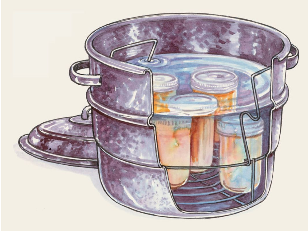
INTERIOR VIEW OF LOADED CANNER. Make sure jars are upright, not touching each other or the sides of the canner, and are covered by at least 1 to 2 inches (2.5 to 5 cm) of water.
